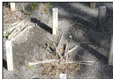
Treated stakes are almost untouched. The untreated control stakes were destroyed.
