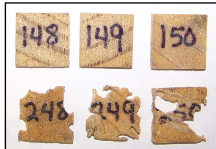
Wood treated with DCOI (top) shows little to no weight loss. Untreated control wood (bottom) shows severe weight loss.
